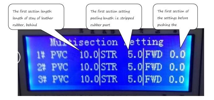
Press the button to start setting, until all the parameters input complete;
