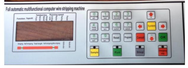
The operation of this system interface consists of a liquid crystal display of 23 buttons and a 192x64 dot matrix composition, each of the following key functions will be introduced:
