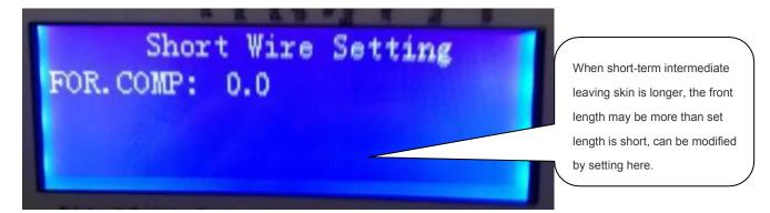
The short-term action sequence: first peeling (front + rear end length length) - > send line (length) - > push skin (back end length) - > cut
