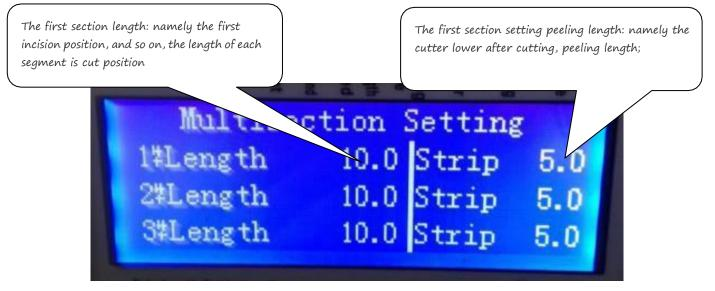
In the non parameter setting state, press, upward or downward view setup parameters of 1-15 segment;
