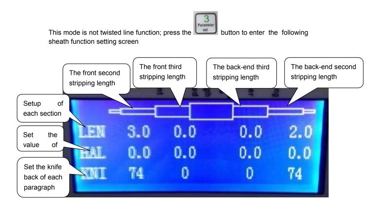
Description: in the sheath model, the program first first peeling, after second times to third times peeling, peeling, so the length of each a skinning knife and value can be
